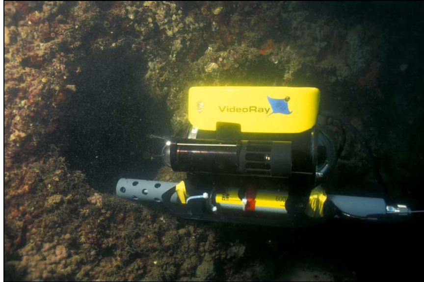
Figure 4.13. VideoRay ROV equipped with YSI Sonde outside on open porthole on USS Arizona 's Second Deck (NPS Photo by Brett Seymour).
